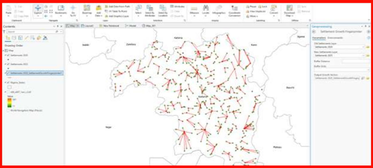
Settlement Growth Finger Tool – Developed a custom Python tool in ArcGIS Pro to analyze and visualize settlement growth patterns. This tool helps stakeholders monitor urban expansion and plan for sustainable development. - A Python tool tested by dummy data based on Kaduna State.
