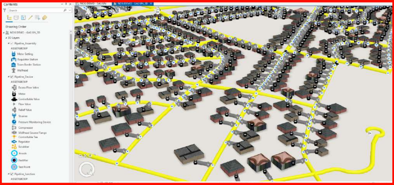
3D Gas Distribution Model – Built a three-dimensional representation of residential gas distribution networks using ArcGIS Utility Network, enabling better visualization of infrastructure and supporting future planning and maintenance workflows. - A Model based on Abuja
